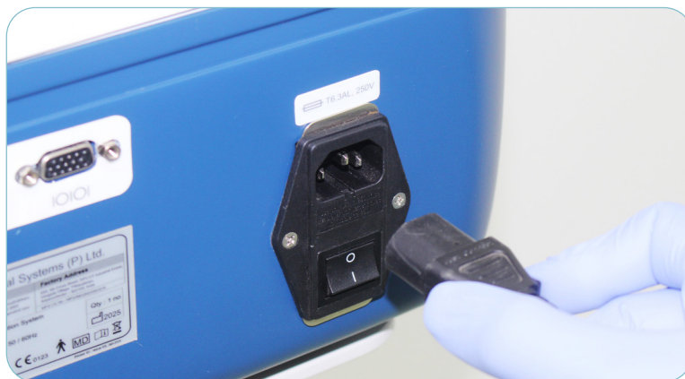
Figure 7.1.A: Connecting power cord into power inlet
