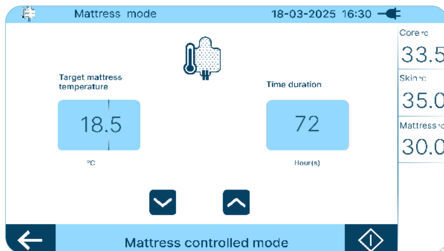
Figure 7.7.2.B: Mattress mode with default parameter settings
