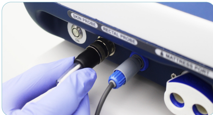
Figure B.1: Connecting skin probe
