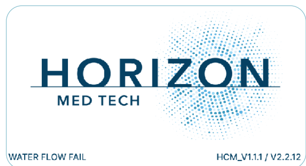
Figure 7.2.B: Start-up screen displaying fail status
