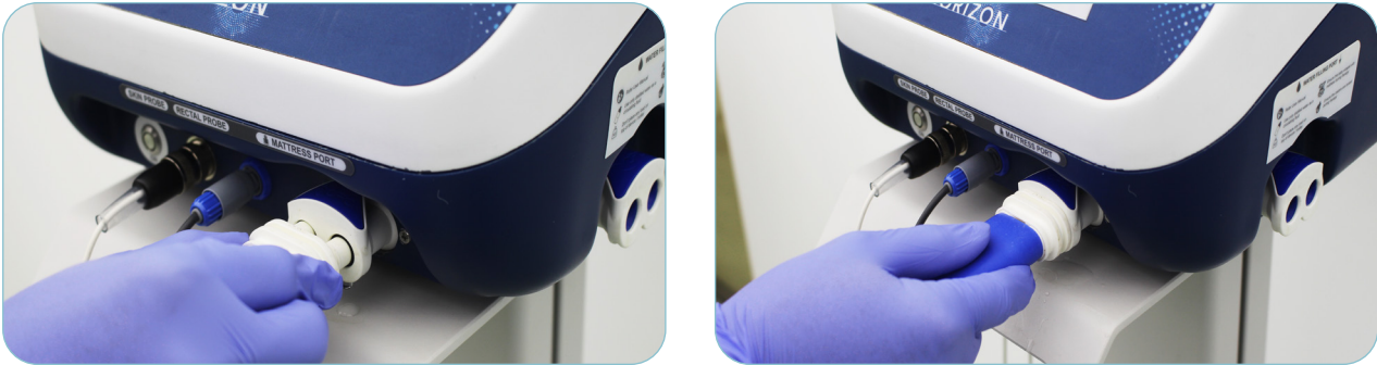
Figure A.1: Long hose connection with head unit
