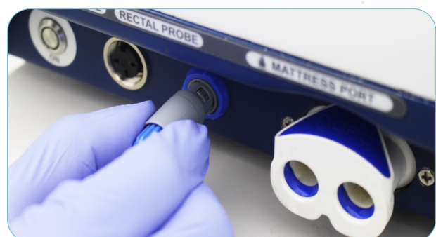
Figure A.2: Connecting rectal temperature probe
