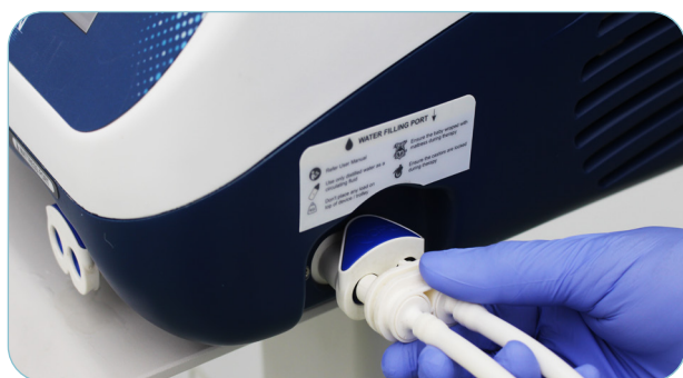
Figure D.1: Filling/Draining bottle connection with head unit
