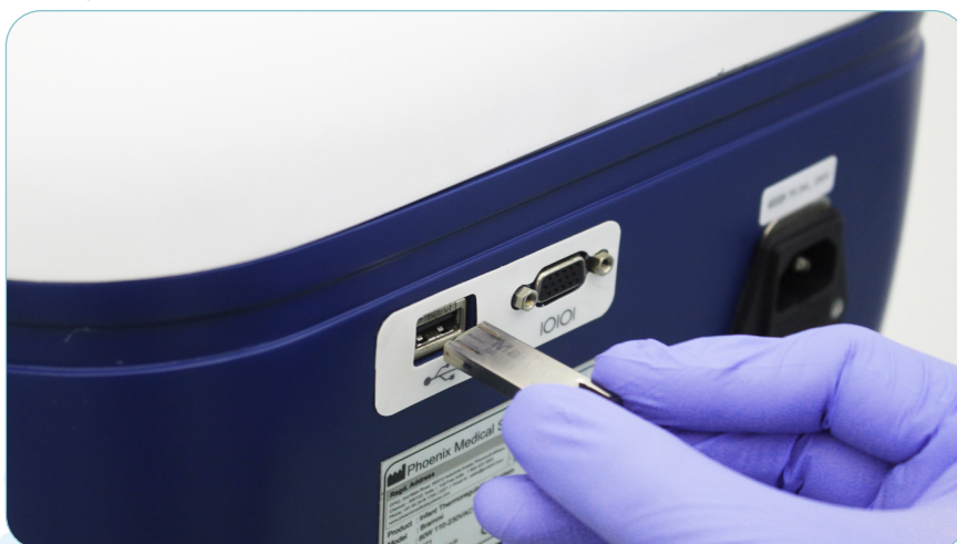
Figure 7.15.B: Connecting USB drive to USB port
