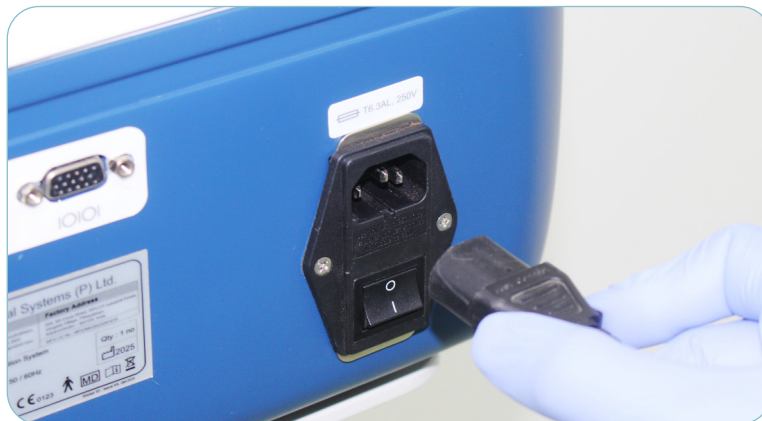
Figure. 7.1.A: Connecting power cord into power inlet
