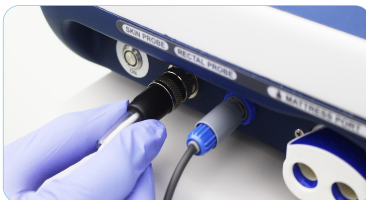
Figure B.1: Connecting skin probe
