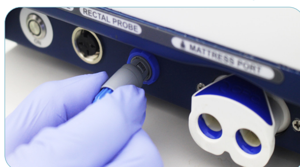
Figure A.2: Connecting rectal temperature probe
