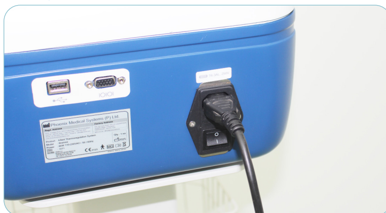
Figure. 7.1.B: Power cord connected
