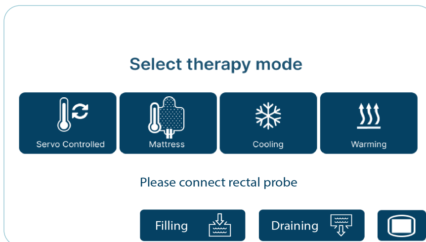
Figure 7.7.3.B: "Please connect rectal probe" displayed when the rectal temperature probe is not connected prior to starting servo therapy
